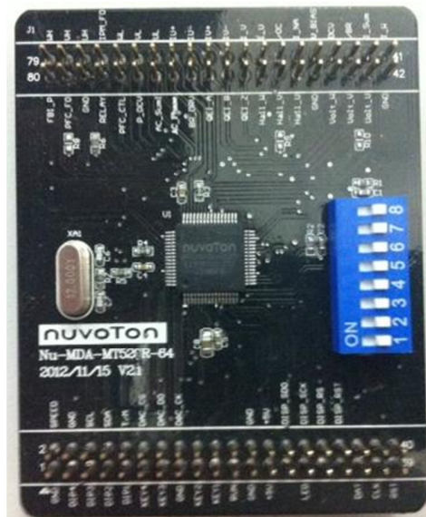
Figure 4-14 Nu-MDA-MT520R-64 Adapter Board Layout
