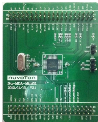
Figure 4-10 Nu-MDA-MINI51 Adapter Board Layout
