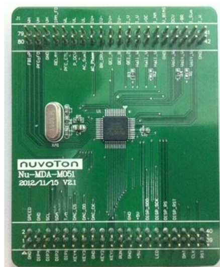
Figure 4-8 Nu-MDA-M051 Adapter Board Layout
